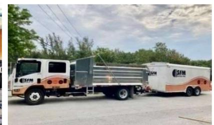
3) Trailer mounted pressure washing rigs equipped with water holding tank & steam pressure capability.
