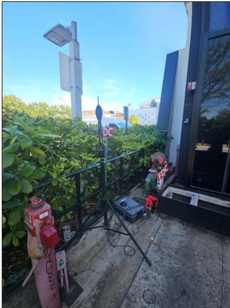
Figure 2. Measurement system and microphone.
