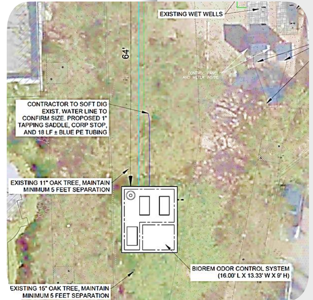
Site plan for job no. L17801 showing proposed location of BIOREM system
