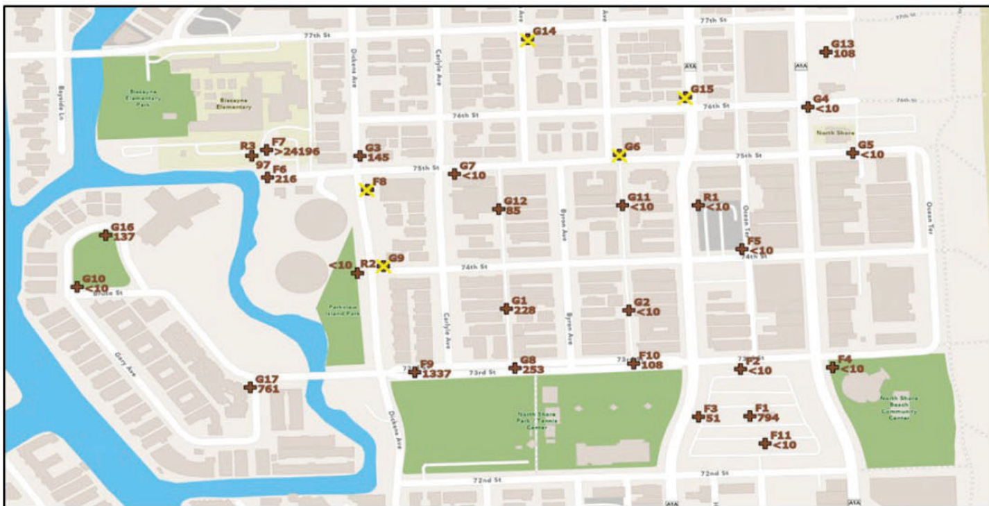
Figure C.1: Groundwater sampling sites. Sites with a yellow “X” were sites that were selected but were found to be non-viable to due excessive underground utilities and were therefore not drilled. The remaining 26 sites without the yellow “X” were sampled. The site ID is given by a “G”, “F”, or “R” (for proximity to gravity sewer, force main, and stormwater conveyance system, respectively) followed by a number. The number below the site ID corresponds to the enterococci concentration in the groundwater in units of MPN/100 mL.
