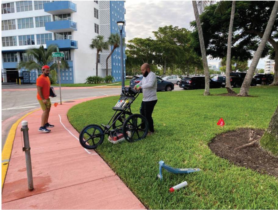
Figure C.13: Illustration of process used to identify underground utilities using ground penetrating radar. The roller device is used to obtain an overall mapping of the utilities and the handheld device (in the foreground on the grass) is used to obtain finer resolution of the underground utilities.
