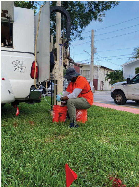
Figure C.14: Illustration of groundwater sample collection from behind the pickup truck mounted drill rig.
