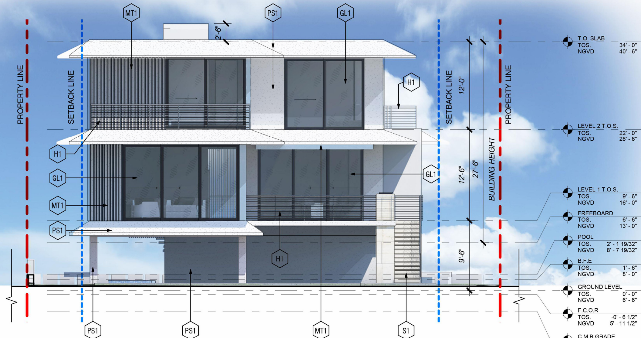
1 EAST ELEVATION 1/8" = 1'-0"
