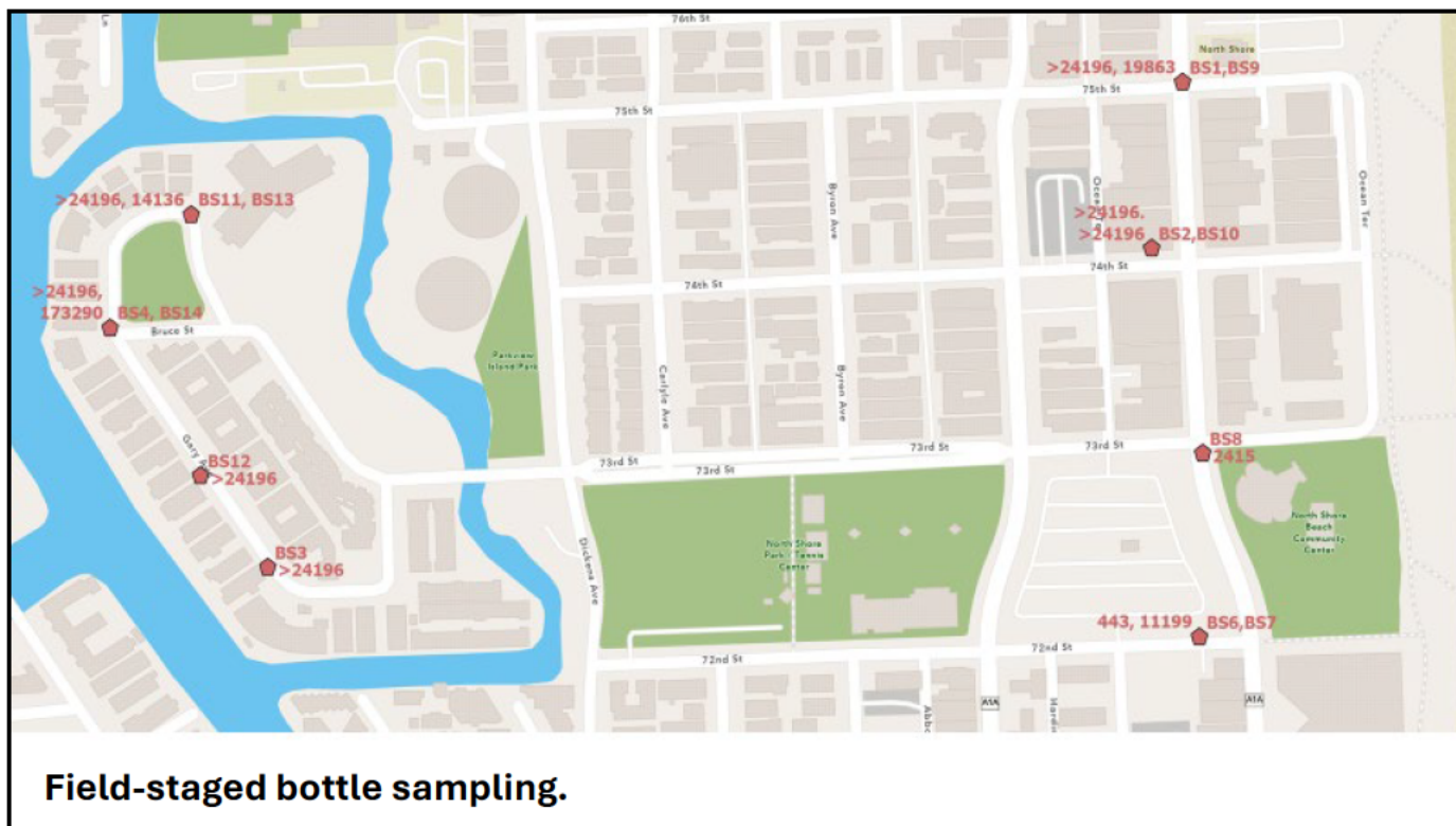
Figure C.3: Field-staged sampling sites. The site ID is given by “BS” followed by a number. The number below the site ID corresponds to the enterococci concentration in the field-staged bottle sample in units of MPN/100 mL.
