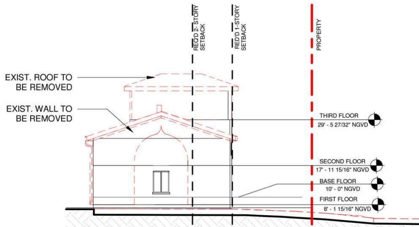
1 DEMOLITION BUILDING 4 PROPOSED SOUTH ELEVATION. 1/16" = 1'-0"
