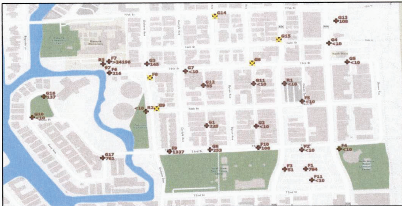
Figure C.1: Groundwater sampling sites. Sites with a yellow “X” were sites that were selected but were found to be non-viable due to excessive underground utilities and were therefore not drilled. The remaining 26 sites without the yellow “X” were sampled. The site ID is given by a “G”, “F”, or “R” (for proximity to gravity sewer, force main, and stormwater conveyance system, respectively) followed by a number. The number below the site ID corresponds to the enterococci concentration in the groundwater in units of MPN/100 mL.
