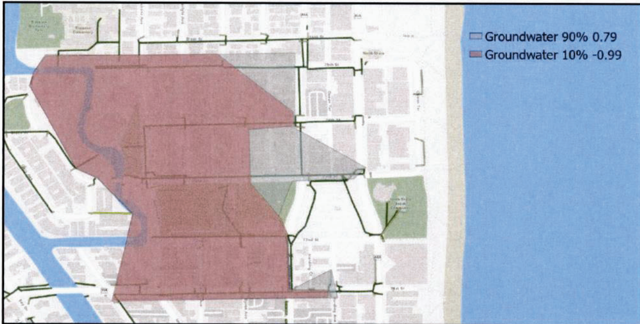
Figure III.5: Stormwater conveyance system with areas of groundwater inundation shown during the lowest 10% elevation (-0.99 ft NGVD) and the highest 90% elevation (0.79 ft NGVD).
