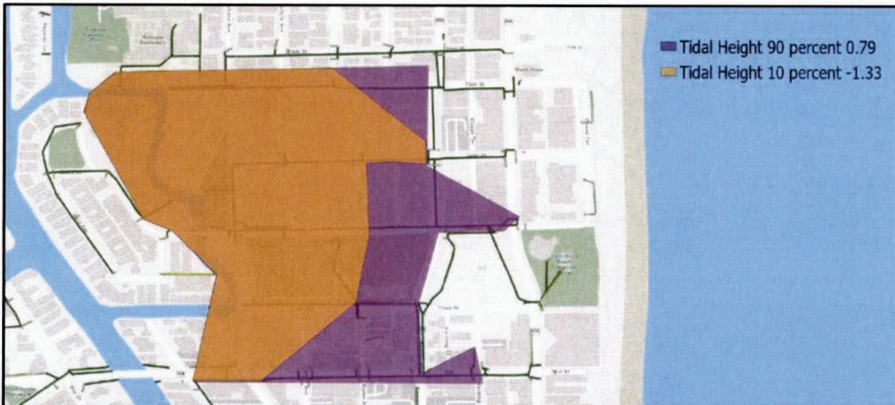
Figure III.6: Stormwater conveyance system with areas of tidal inundation shown during the lowest 10% elevation (-1.33 ft NGVD) and the highest 90% elevation (0.79 ft NGVD). The reference for the tidal data is the NOAA station located on Virginia Key at Bear Cut.
