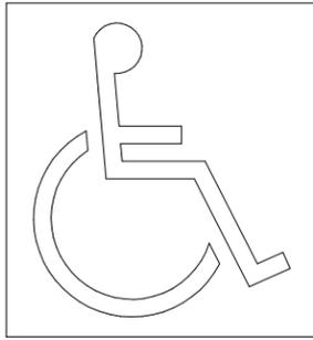
THIS SYMBOL TO BE PAINTED ON THE HORIZONTAL PAVED SURFACE OF ACCESSIBLE SPACES WHERE REQUIRED BY LOCAL ORDINANCES. COLOR TO BE IN CONTRAST WITH THE BACKGROUND. SIZE TO BE ACCORDING TO STATE CODE.
