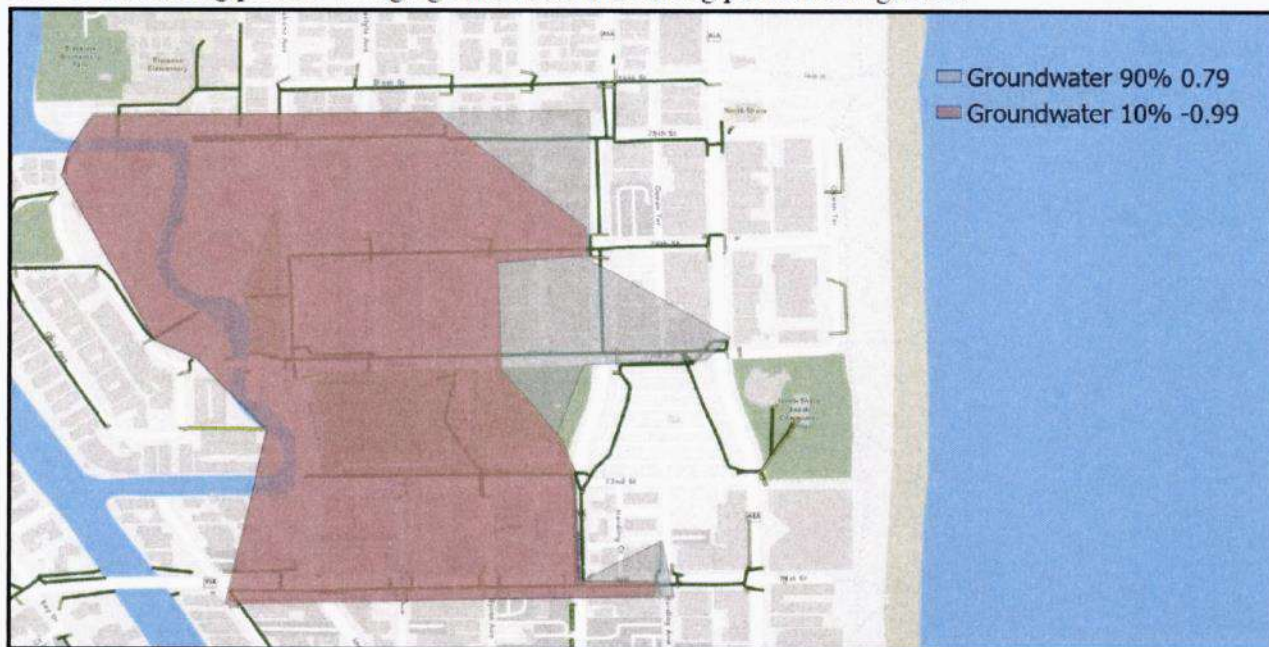
Figure III.5: Stormwater conveyance system with areas of groundwater inundation shown during the lowest 10% elevation (-0.99 ft NGVD) and the highest 90% elevation (0.79 ft NGVD).
