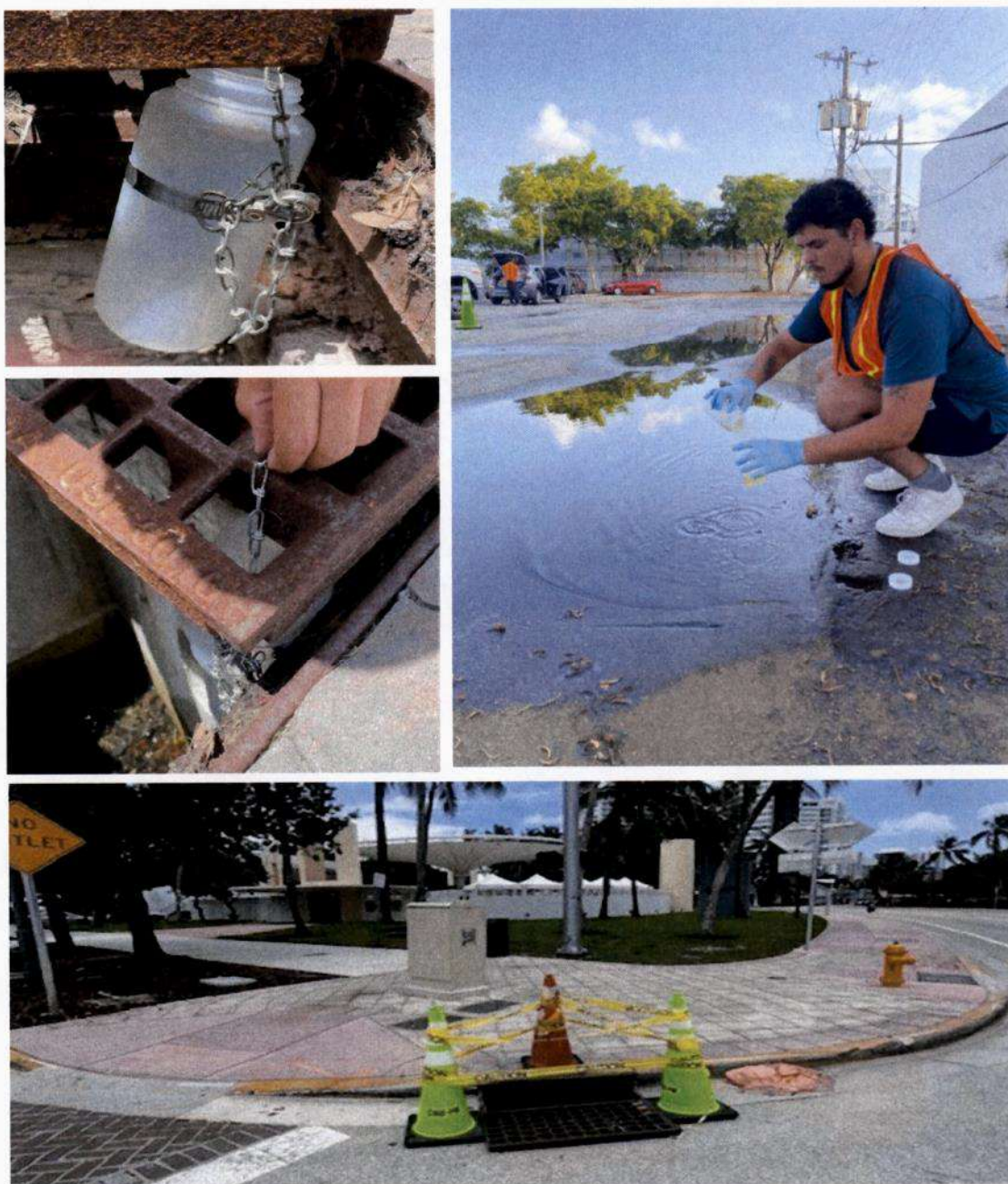
Figure C.15: Illustration of stormwater sampling. Top two square photos illustrate the field-staged bottle sample set up hanging immediately below the catch basin grate. Top right photo illustrates puddle sampling. The bottom photo illustrates the set up for in-person runoff sampling requiring the removal of the top grate or manhole cover for manual placement of a bottle to collect water as it falls into the catch basin.
