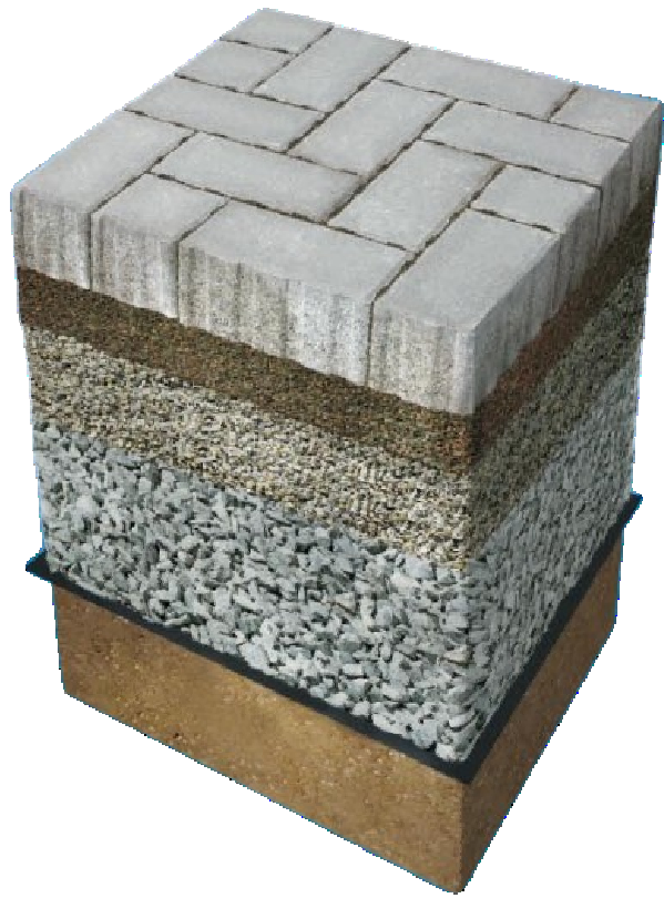
PAVER INSTALLATION DETAIL
