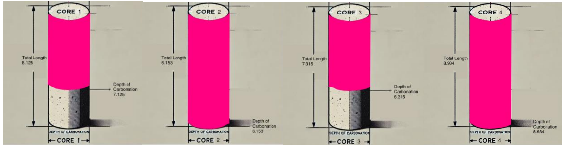
Figure 1- Depth of Carbonation (Core 1) Figure 2- Depth of Carbonation (Core 2) Figure 3- Depth of Carbonation (Core 3) Figure 4- Depth of Carbonation (Core 4)
