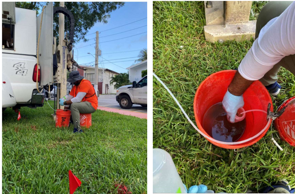
Figure C.14: Illustration of groundwater sample collection from behind the pickup truck mounted drill rig.
